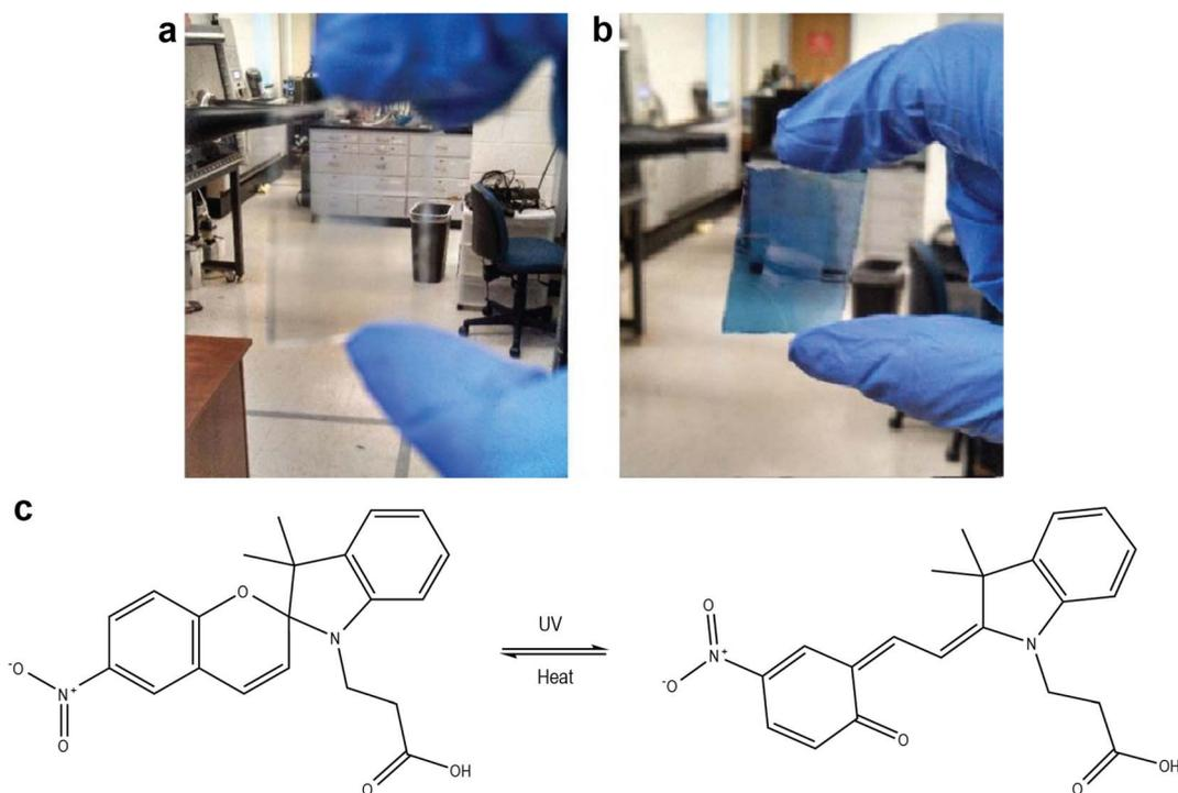
Fig. 4 Color change of a spirooxazine dye on a TiO<sub>2</sub> film (a) before and (b) after exposure to sunlight. DSCs fabricated using this dye showed power conversion efficiencies of 0.007% (clear) and 0.028% (colored). (c) Chemical structures of the dyes shown above. Figure adapted with permission from ref. 31. Copyright 2015 by Johnson et al., licensee AIMS Press.
