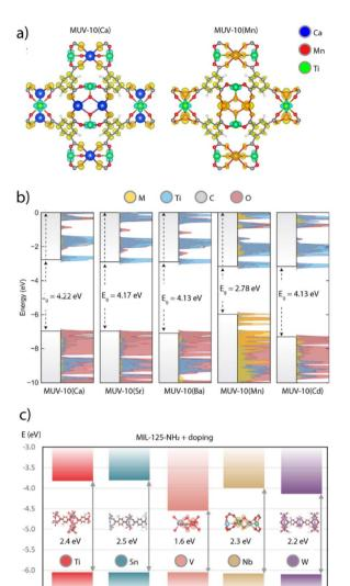
Fig. 5 (a) Electron density in the VB (yellow) and CB (red) of MUV-10(Ca) and MUV-10(Mn) frameworks. (b) Density functional theory DOS calculations for all MUV-10(M) derivatives showing the impact of metal node modification in their theoretical band gaps. (c) Calculated impact of metal doping in the theoretical band gap of MIL-125-NH<sub>2</sub>. Adapted from ref. 41, 86 and 89.
