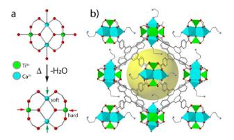
Fig. 7 (a) Scheme illustrating the generation of hard and soft open metal sites in the heterometallic Ti<sub>2</sub>Ca<sub>2</sub> clusters by thermal desolvation of MUV-10. (b) Simulated structure of MUV-12-DAP showing the selective grafting of diamines to vacant Ca<sup>2+</sup> sites. Adapted from ref. 87.
