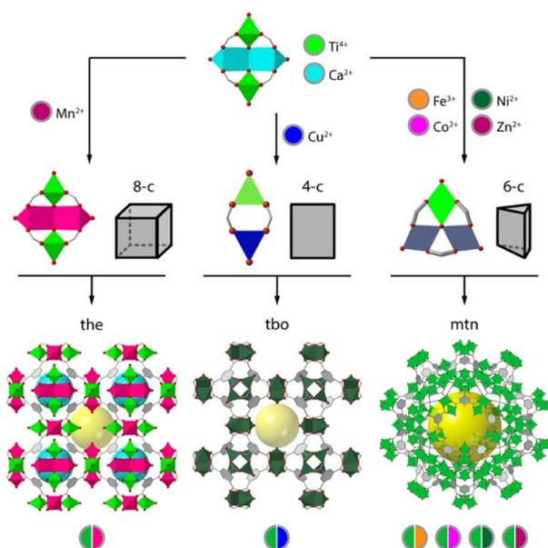
Fig. 4 Metal-exchange reactions with the  $\text{Ti}_2\text{Ca}_2$  clusters in MUV-10 lead to heterobimetallic titanium frameworks of varying connectivity and chemical composition, which results in the formation of the corresponding net topologies all fixed by the identity of the incoming metal.
