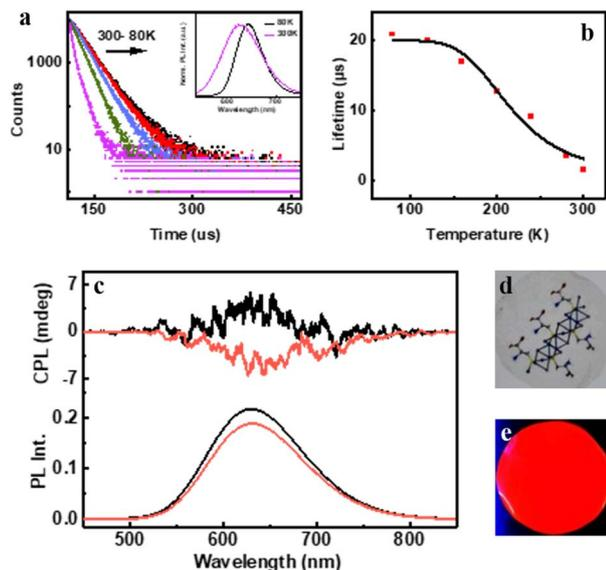
Fig. 5 (a) Temperature dependent lifetime decay for the PVA film incorporated with  $(D-Cys)_2Cu_4I_4$ . Inset shows the normalised PL spectra at 80 K and room temperature. (b) PL lifetime decay vs. temperature plot fitted with the Boltzmann equation. (c) CPL (top) and PL (bottom) spectra from the films prepared using  $(D-Cys)_2Cu_4I_4$  (black trace) and  $(L-Cys)_2Cu_4I_4$  (red trace) nanoclusters. Photographs of the film under (d) visible and (e) UV light illumination.
