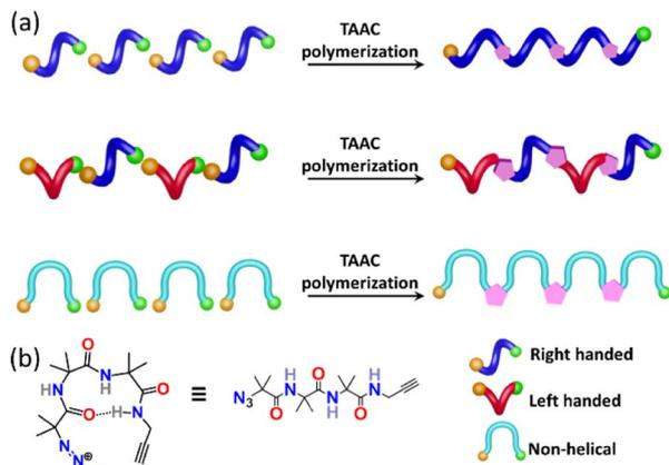
Fig. 1 Design of a  $\beta$ -turn forming monomer that can form polymorphs via adopting various  $\beta$ -turn conformations. (a) Schematic showing plausible conformations of azide–alkyne modified  $\beta$ -turns in various polymorphic forms and their TAAC polymerization to yield polymorphs of a polymer. Azide and alkyne are represented as orange and green balls, respectively. (b) Chemical structure of the designed tripeptide **1**.
