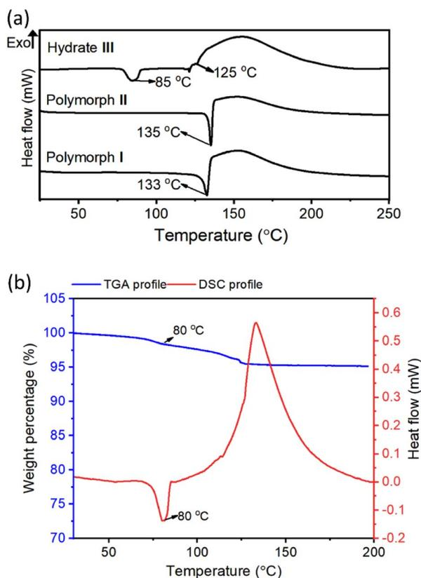
Fig. 3 Thermal analysis of monomers. (a) DSC profiles for crystals of the polymorphs I and II, and the hydrate III at a heating rate of 5 °C min<sup>-1</sup>. (b) Comparison of DSC and TGA profiles of hydrate III crystals recorded at a heating rate of 1 °C min<sup>-1</sup>.
