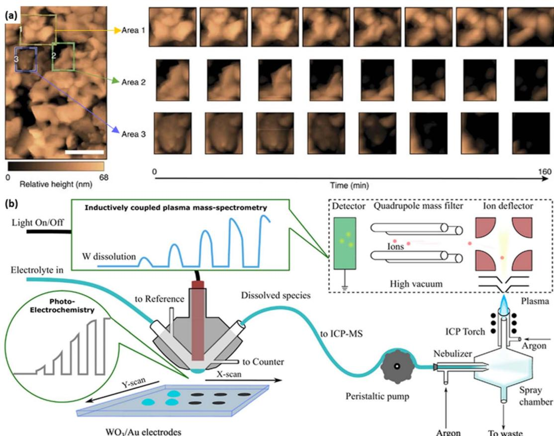
Fig. 6 (a) *In situ* EC-AFM images of the BiVO<sub>4</sub> photoanode. Three coloured boxes represent area 1 (yellow), area 2 (green) and area 3 (blue), of which *operando* scans are recorded in detail. Reprinted with permission from ref. 67, copyright 2016, Nature Publishing Group. (b) Schematic combination of the inductively coupled plasma mass spectrometry (ICP-MS) and the illuminated scan flow cell (SFC). Reprinted with permission from ref. 71, copyright 2018 Elsevier B.V.
