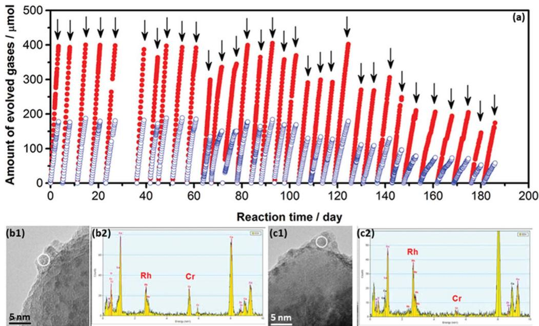
Fig. 4 (a) Long-term measurement of  $\text{Rh}_{2-y}\text{Cr}_y\text{O}_3/\text{GaN}:\text{ZnO}$  photocatalyst for overall water splitting under visible light. (b and c) Combination of TEM and EDS analysis for the  $\text{Rh}_{2-y}\text{Cr}_y\text{O}_3/\text{GaN}$  photocatalyst (b) before and (c) after deactivation. Reproduced from ref. 51, copyright 2012, American Chemical Society.
