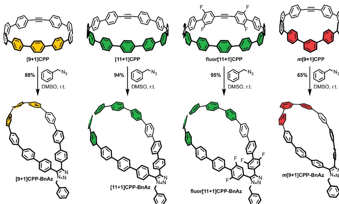
Scheme 3 Strain-promoted azide–alkyne cycloaddition reactions between the  $[n+1]$ CPPs described in this study and benzyl azide, a model compound. Yields were determined *in situ* *via* quantitative <sup>1</sup>H NMR in comparison to an internal standard, dimethyl sulfone.
