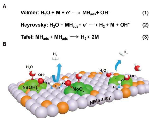
**Fig. 1** (A) The reaction mechanism for the HER in alkaline electrolytes and two pathways are presented in the forms of the Volmer–Heyrovsky mechanism and the Volmer–Tafel mechanism. (B) Schematic diagram of synergistic catalysis of alloy–oxide or alloy–hydroxide interface structures, in which the oxide or hydroxide promotes water dissociation and the alloy accelerates hydrogen combination.
