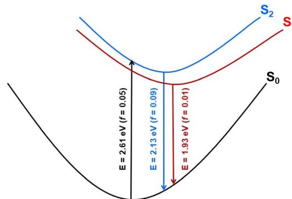
Fig. 8 Schematic potential energy profiles of the lowest excited states of **8H** constructed on the basis of theoretical results. Vertical arrows illustrate vertical absorption from the ground state (black) and fluorescence (blue and red) from the lowest excited singlet states with values of transition energy ( $E$ ) and oscillator strength ( $f$ ) computed at the ADC(2)/cc-pVDZ theoretical level.
