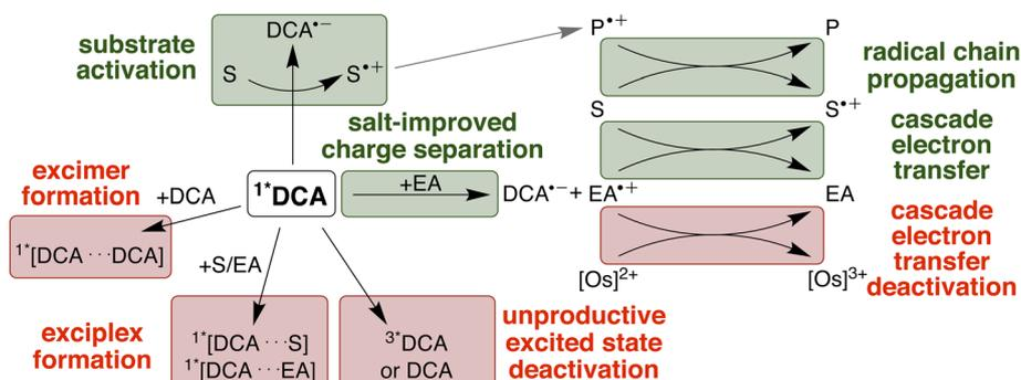
Fig. 7 Summary of productive and unproductive pathways for the deactivation of  $^1DCA$  after triplet–triplet annihilation upconversion. EA = electron acceptor/mediator; S = substrate; P = product. Favourable processes are coloured in green, unwanted processes in red.
