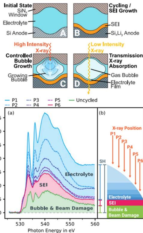
Fig. 5 (a) Illustration of a novel approach to investigate the SEI on silicon thin-film electrodes *in situ* through transmission sXAS and (b) extraction of the SEI spectrum from the overshadowing electrolyte spectrum and subtraction of the bubble and beam damage.<sup>82</sup>
