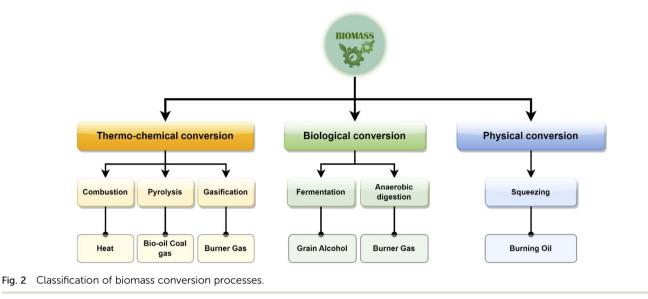
biomass-to-syngas production systems. The classification of biomass conversion is shown in Fig. 2.
