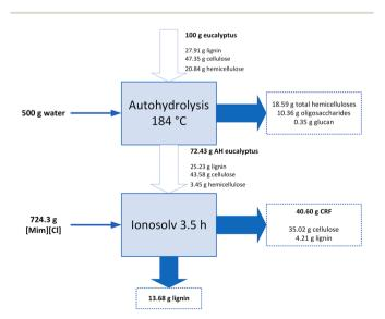
Fig. 4 Mass balance per  $100~{\rm g}$  of eucalyptus wood at the optimum combined process conditions.
