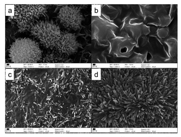
Fig. 3 SEM micrographs of hentriacontane-14,16-dione recrystallized by different solvents, (a) petroleum ether, (b) toluene, (c) TMO, and (d) DEDMO. Scale bars: 1 µm.
