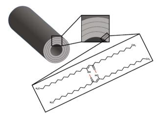
Fig. 5 Proposed model of a nano-structure tubule composed of layers of  $\beta$ -diketone according to Jetter et al.<sup>44</sup> and Ensikat et al.<sup>70</sup>
