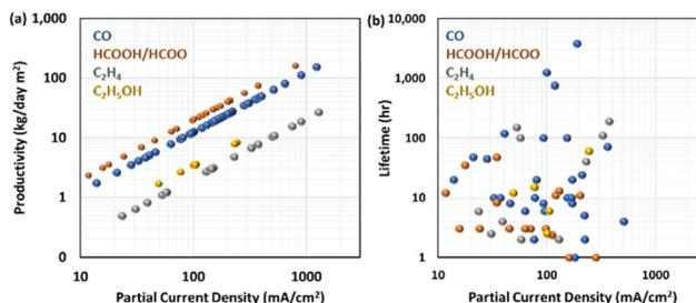
**Fig. 6** (a) The expected production rate per day as a function of the partial current density for each CO<sub>2</sub>RR product with the experimental data according to the literature survey. (b) Reported lifetime of CO<sub>2</sub>RR as a function of the partial current density for each CO<sub>2</sub>RR product with the experimental data according to the literature survey.
