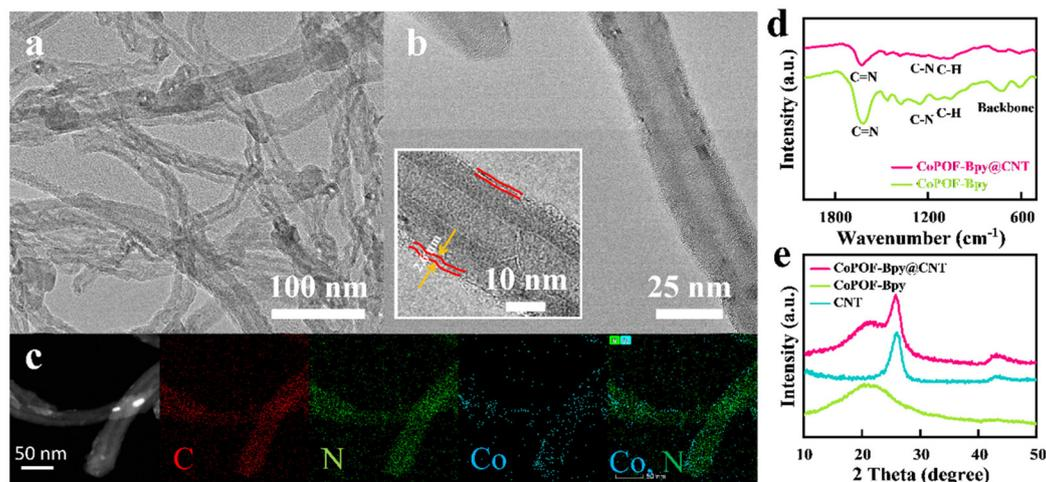
**Fig. 1** (a) TEM image of CoPOF-Bpy@CNT; (b) HR-TEM image of CoPOF-Bpy@CNT, and the inset is the enlarged view; (c) the corresponding EDX mapping of CoPOF-Bpy@CNT; (d) FT-IR spectra and (e) XRD patterns of CoPOF-Bpy@CNT and CoPOF-Bpy.
