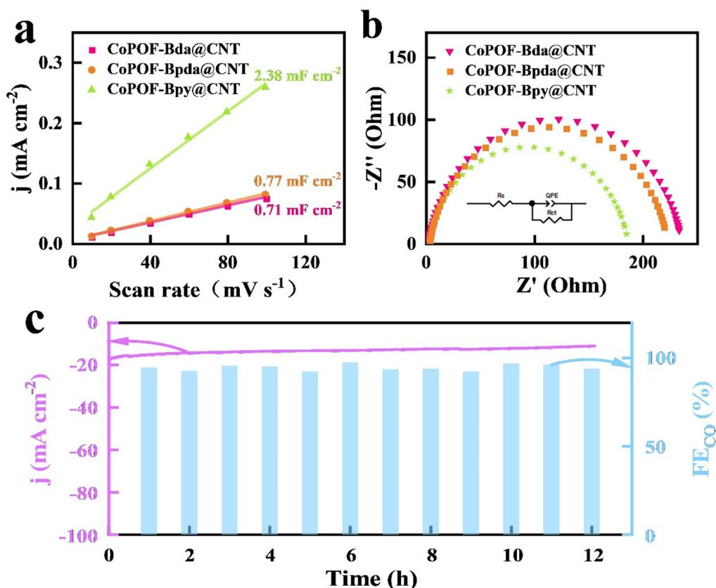
**Fig. 4** (a)  $C_{dl}$  values of CoPOF-Bpy@CNT, CoPOF-Bda@CNT, and CoPOF-Bpda@CNT in the non-faradaic region with various scan rates (10–100  $\text{mV s}^{-1}$ ); (b) Nyquist plots by EIS; (c) measurements for assessing the long-term stability of CoPOF-Bpy@CNT at  $-0.7$  V vs. RHE in a  $\text{CO}_2$ -saturated 0.5 M  $\text{KHCO}_3$  solution for 12 h.
