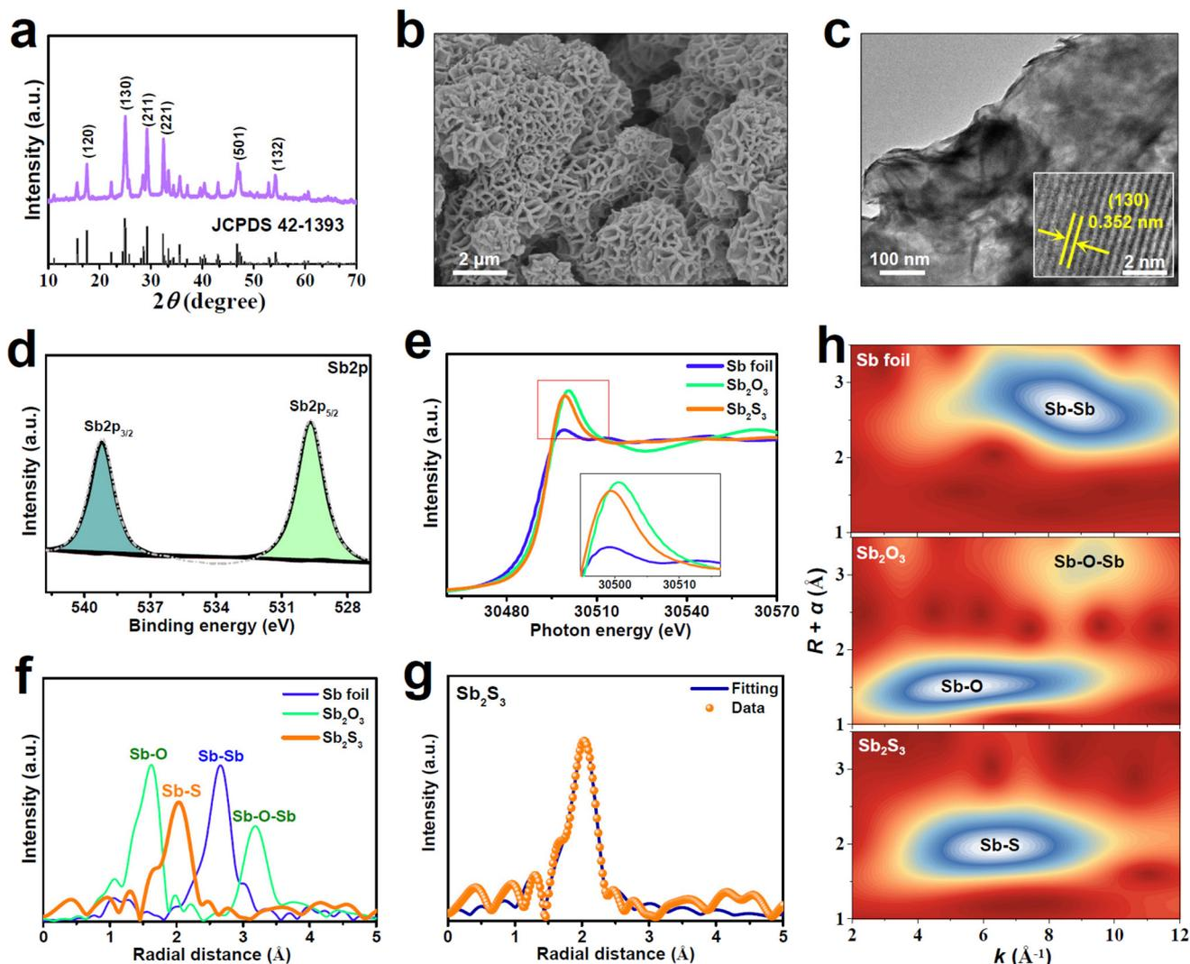
**Fig. 1** Characterization of  $\text{Sb}_2\text{S}_3$ : (a) XRD pattern, (b) SEM image, (c) TEM image and HRTEM image (inset), (d) XPS  $\text{Sb}2p$  spectrum, (e)  $\text{Sb}$  K-edge XANES spectra, (f) EXAFS spectra and (h) WT profiles of  $\text{Sb}_2\text{S}_3$  and reference samples. (g) EXAFS fitting curve of  $\text{Sb}_2\text{S}_3$ .
