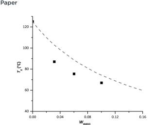
**Fig. 7** Evolution of experimental (square) and theoretical (dashed line)  $T_{\rm g}$  with the mass fraction of BMDO. Theoretical values were calculated with the Fox equation.
