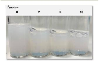
**Fig. 4** Photos of the latexes prepared with different initial molar fraction of BMDO. From left to right: experiments E1MMA,  $f_{\rm BMDO,0}=0\%$ ; E4BMDO,  $f_{\rm BMDO,0}=2\%$ ; E1BMDO,  $f_{\rm BMDO,0}=5\%$ ; E5BMDO,  $f_{\rm BMDO,0}=10\%$  (Table 1).
