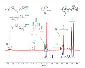
Fig. 2 <sup>1</sup>H NMR spectra of the dried extract of latexes E1BMDO (red) and E1MMA (blue) (CDCl<sub>3</sub>, 256 scans). Assignments were made according to a previous report.<sup>13</sup> B stands for BMDO units and M for MMA units in a triad. D2 corresponds to one of the identified degradation products of BMDO (see ESI, Fig. S1†).
