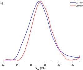
**Fig. 3** (a) SEC traces from the UV detector obtained for the dried extract from experiments E1MMA ( $f_{\rm BMDO,0}=0\%$ ) and E1BMDO ( $f_{\rm BMDO,0}=5\%$ , Table 1), normalized on the maximum of absorption. (b) SEC traces from the UV detector set at 217 nm (blue) and 260 nm (red) obtained for experiment E1BMDO (Table 1).
