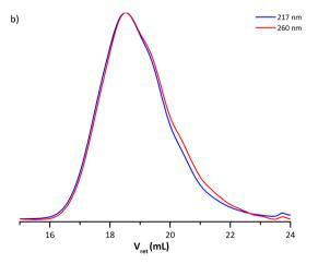
**Fig. 5** (a) Molar mass distributions of dry extracts for latexes E4BMDO (red), E5BMDO (blue), E1BMDO (green) and EMMA1 (black) (Table 1). (b) UV chromatograms from SEC-THF analysis at 217 nm (blue) and 260 nm (red) for the dried latex E5BMDO.
