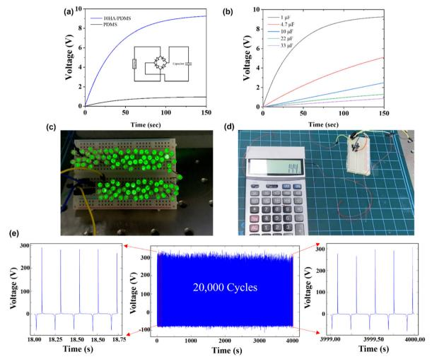
Fig. 5 (a) The charging curves of a 1 µF capacitor comparing PDMS and optimal 10HA/PDMS at an input frequency of 5 Hz and an applied force of 2 N. (b) The charging curves of different capacitors with optimized 10HA/PDMS at an applied force of 2 N. (c and d) HA-TENG powering 100 LEDs or a commercial calculator. (e) Endurance test of the optimized HA-TENG for more than 20 000 cycles.
