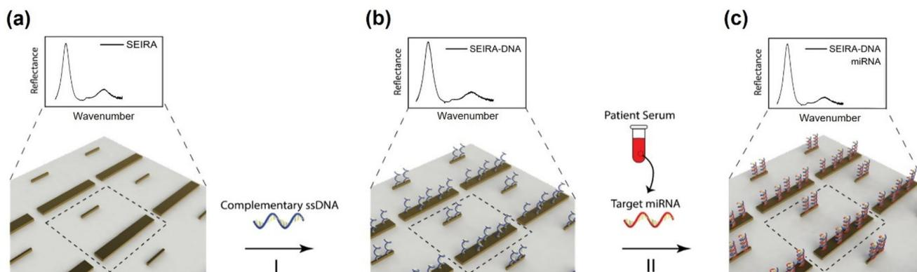
**Fig. 2** Experimental workflow. (a) Measurement was performed on a clean SEIRA sensor (zoom-in view). Dashed square is a design unit cell of the SEIRA structure. (b) Step I: Complementary ssDNA (with thiol group modification) solution was immobilized onto the SEIRA substrate. Measurement was performed on the SEIRA-DNA substrate. (c) The total RNA solution containing target miRNA molecules was immobilized onto the SEIRA-DNA substrate. Measurement was performed on the SEIRA-DNA-miRNA substrate.
