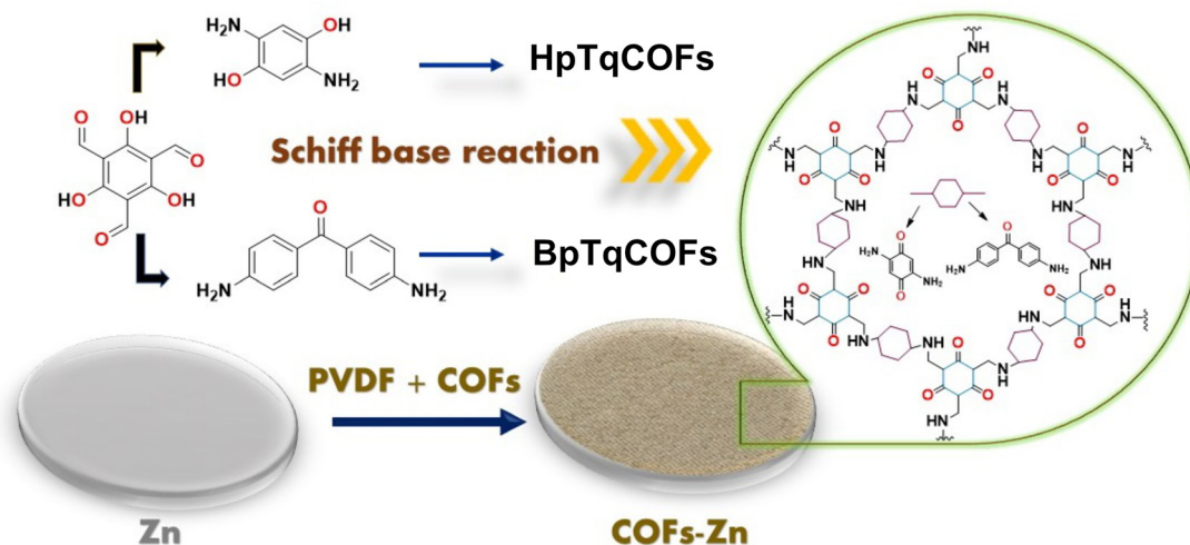
Fig. 1 Scheme of structures and the preparation of COF layers: HqTpCOF and BpTpCOF as ASEIs on the Zn anode in AZIBs.
