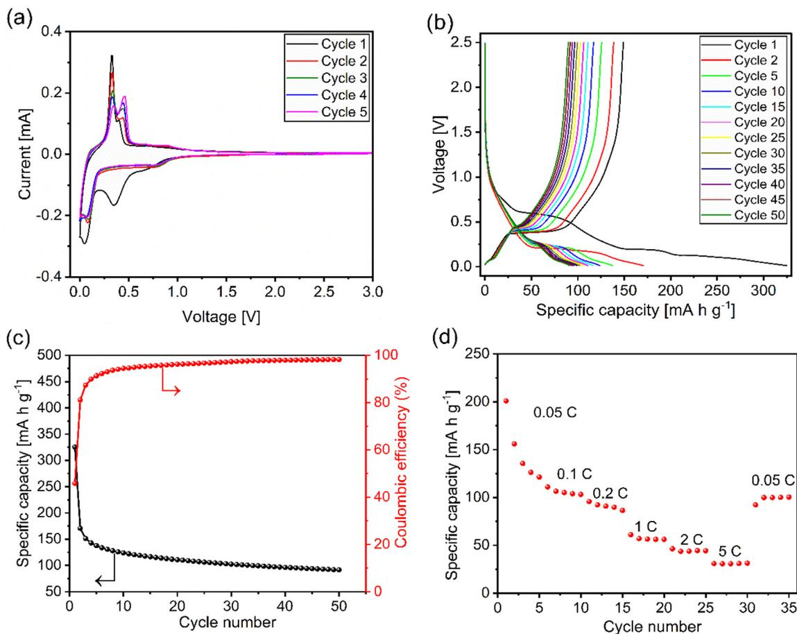
**Fig. 5** Electrochemical performance of NTO electrodes (a) cyclic voltammogram curves in a voltage range of 0.0–3.0 V at a scanning rate of  $0.08 \text{ mV s}^{-1}$ , (b) charge–discharge profiles in a voltage range of 0.01–2.5 V at current density of  $10 \text{ mA g}^{-1}$ , (c) cycling performance of NTO electrode at current density of  $10 \text{ mA g}^{-1}$  (d) rate capability of NTO electrode.
