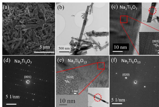
**Fig. 3** (a) SEM image of the mixed phase rods, (b) low-resolution TEM image of the rods, (c) HRTEM image of a  $\text{Na}_2\text{Ti}_3\text{O}_7$  rod with inset low-resolution image and one to resolve lattice fringes, (d) corresponding SAED pattern, (e) HRTEM image of a  $\text{Na}_2\text{Ti}_6\text{O}_{13}$  rod with low-resolution inset image to resolve lattice fringes, (f) corresponding SAED pattern.
