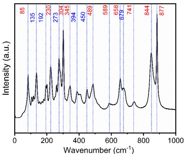
**Fig. 2** Raman spectrum of NTO sample, the red arrows correspond to the  $\text{Na}_2\text{Ti}_3\text{O}_7$  phase and blue arrows  $\text{Na}_2\text{Ti}_6\text{O}_{13}$ .
