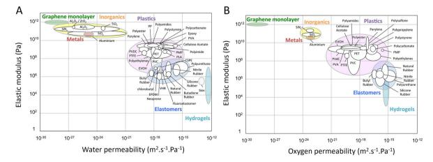
Fig. 6 The water and oxygen permeability of different materials.<sup>179</sup> Copyright 2018, American Chemical Society
