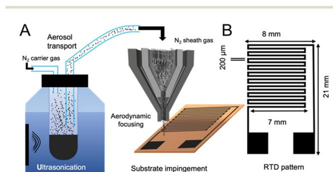
**Fig. 1** Aerosol jet printing resistive temperature sensors. (A) Schematic depicting the steps of aerosol jet printing including the ultrasonication, transport, aerodynamic focusing and substrate impingement. (B) The geometry of the RTD sensors designed to be printed.
