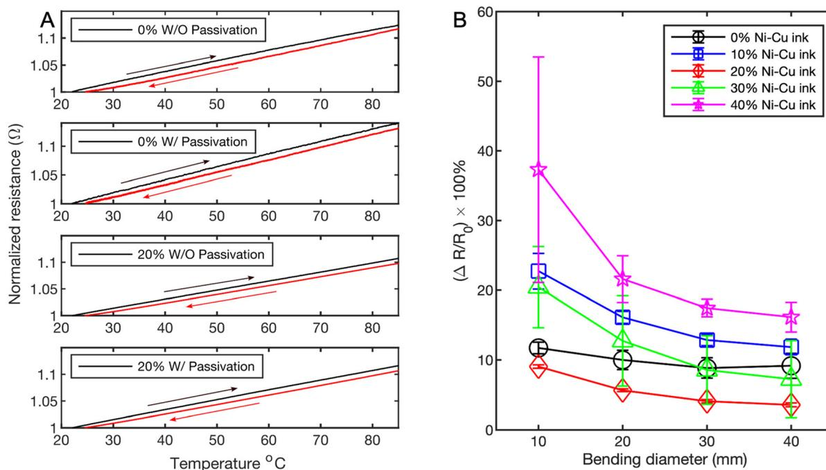
**Fig. 6** Effect of passivation and bending strain on aerosol jet printed temperature sensors with hybrid inks. (A) Temperature cycling test for sensors printed with 0% and 20% Ni-Cu ink with and without Polyimide passivation, RH = 75%. (B) Normalized resistance change percentage with respect to different bending diameter for sensors printed with different hybrid inks.
