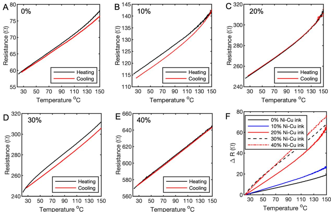
**Fig. 4** Resistance-temperature measurement results for resistive temperature sensors aerosol jet printed with various inks both for heating and cooling cycles. Various hybrid inks with added Ni–Cu ink volumetric percentages ranging from 0% to 40% are measured and displayed as follows: (A) 0% Ni–Cu ink (B) 10% Ni–Cu ink, (C), 20% Ni–Cu ink, (D) 30% Ni–Cu ink, (E) 40% Ni–Cu ink. (F) Comparison of resistance change with respect to temperature for various inks.
