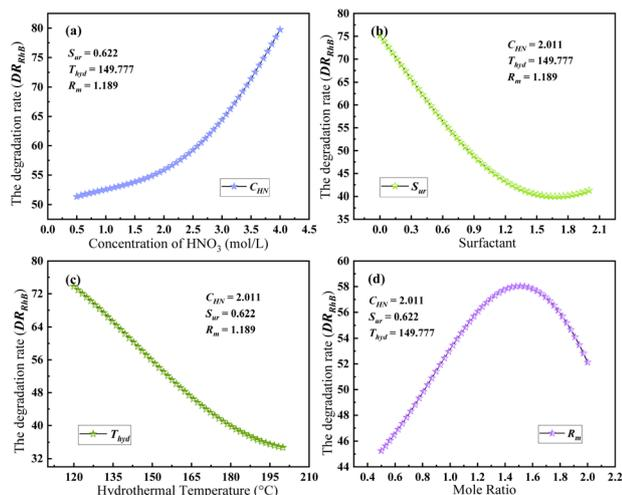
Fig. 9 SA of the four features based on the SVR-RBF model (a)  $C_{\text{HN}}$ , (b)  $S_{\text{ur}}$ , (c)  $T_{\text{hyd}}$  and (d)  $R_{\text{m}}$ .
