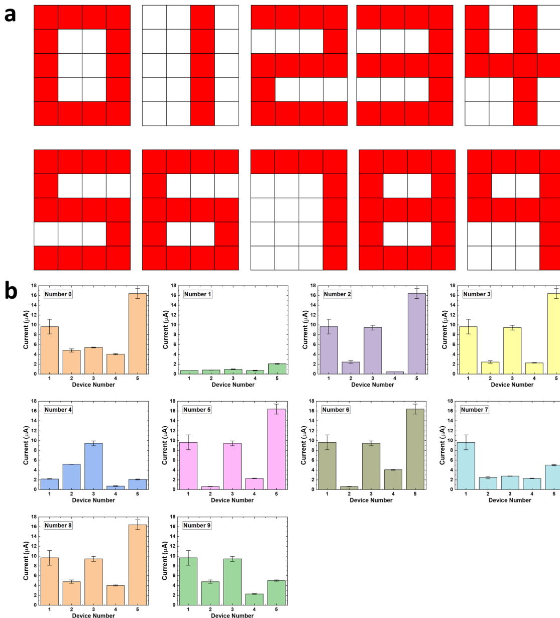
Fig. 5 (a) Images of 10 numbers used in this test. (b) Measured reservoir states after the memristors are subjected to the 10 inputs. The reservoir states are reflected as the read currents of the 5 memristors forming the reservoir.
