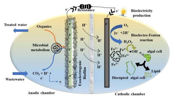
Fig. 1 Schematic diagram of a bio-electro-Fenton-assisted photosynthetic microbial fuel cell.
