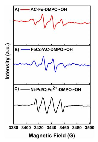
Fig. 6 The EPR spectra of (A) AC-Fe, (B) FeCo/AC, and (C) Ni-Pd/C-Fe<sup>2+</sup> using DMPO as the trapping reagent.
