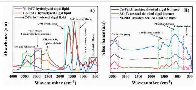
Fig. 9 (A) The FTIR spectra of algal lipid; and (B) lipid extracted de-oiled algal biomass.
