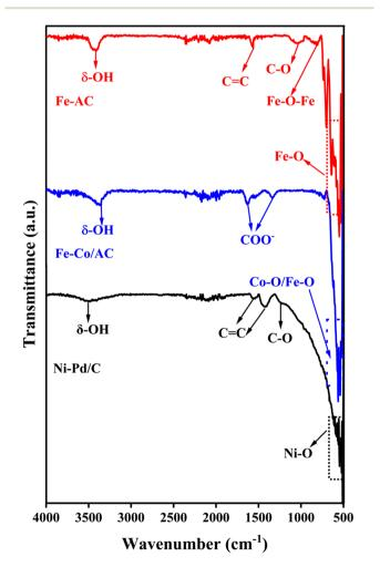
**Fig. 3** The FTIR spectrum of AC-Fe (red); CoFe-AC (blue); and Ni-Pd/C (black) catalysts with the respective functional groups.
