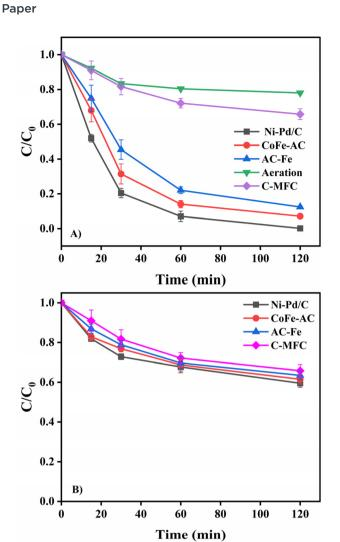
Fig. 5 Degradation of methylene blue (A) without, and (B) with the addition of 2-propanol.
