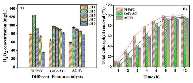
Fig. 7 (A) Variation of different  $H_2O_2$  concentrations produced by employing different catalysts under the pH range from 1.0 to 9.0; (B) total chlorophyll removal (%) during the different time intervals.
