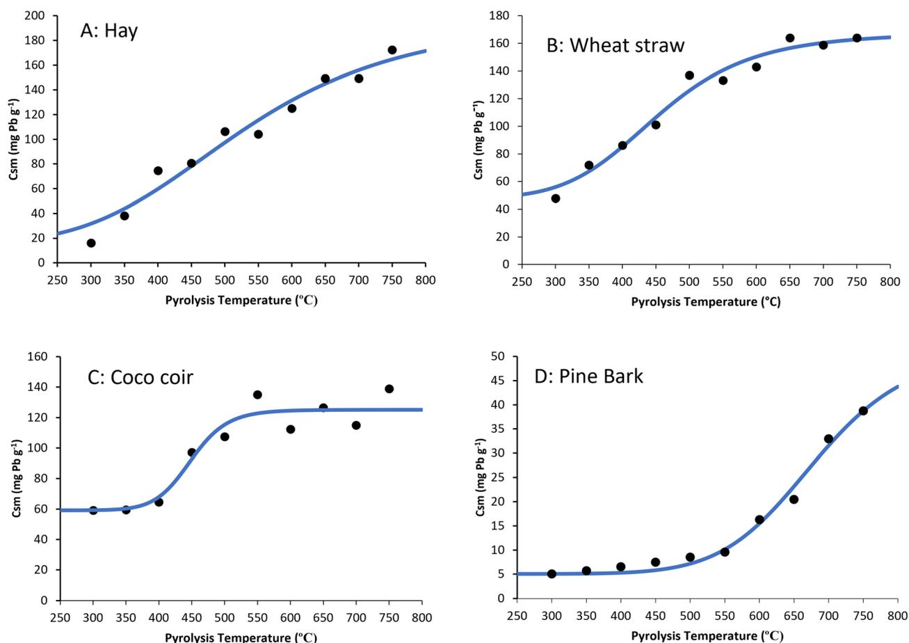
**Fig. 1** Relationship between Pb sorption capacity and biochar pyrolysis temperature. Pb maximum sorption capacity ( $C_{sm}$ ) of hay (A), wheat straw (B), coco coir (C), and pine bark (D) biochars plotted against pyrolysis temperature and fitted to a sigmoidal model that quantifies the relationship.
