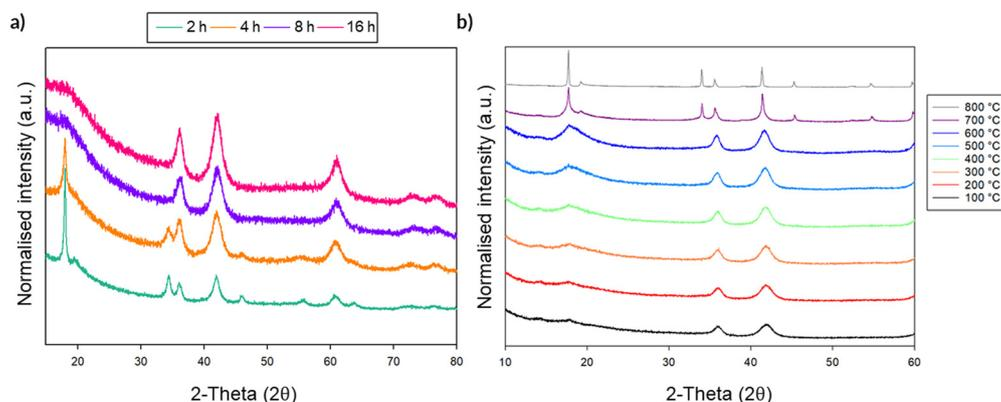
Fig. 12 (a) PXRD of  $\text{Li}_2\text{SnO}_3$  with increasing mill time. Conversion to DRS occurs at  $\sim 8 \text{ h}$  (b) Plot showing the changes in PXRD pattern with increasing temperature, showing the transformation from DRS to layered on heating. (Cu  $K\alpha$ ).
