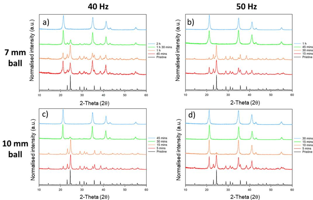
Fig. 6 Resulting PXRD patterns from the study of ball mill frequency, time and ball size on the milling of  $\text{Li}_2\text{MoO}_4$ . Patterns (a) and (b) made use of a 7 mm ball at 40 Hz and 50 Hz, respectively. Patterns (c) and (d) made use of a 10 mm ball at 40 Hz and 50 Hz respectively. The conversion rate was shown to significantly reduce with lower frequency or ball size. (Cu  $K\alpha$ ). 50 mg of material was loaded into the pots in each case.
