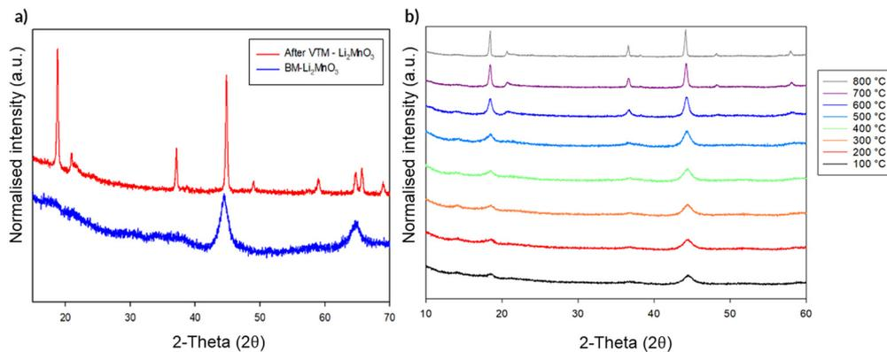
Fig. 11 (a) PXRD of BM- $\text{Li}_2\text{MnO}_3$  sample before (DRS phase) and after VT-PXRD (layered phase) (b) VT-PXRD experiment in the region of 100–800 °C showing the change in the relative intensity of peaks with increasing temperature indicating a transformation from DRS to layered on heating. (Cu  $K\alpha$ ).
