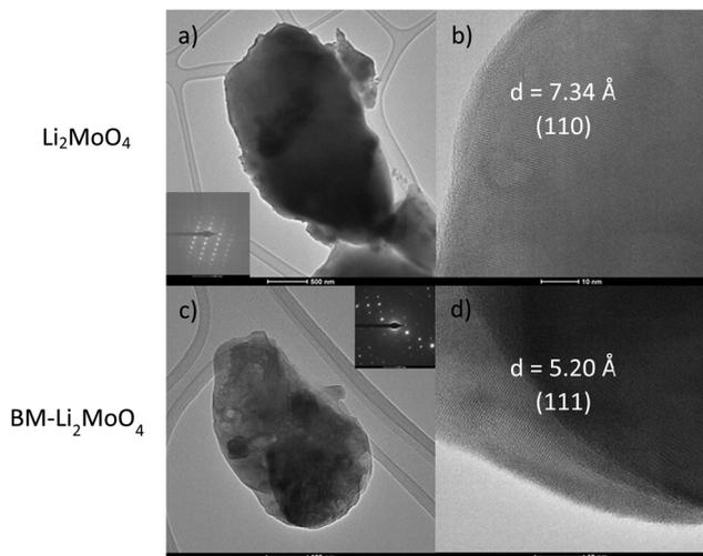
Fig. 4 TEM images of pristine (a) and ball milled (c)  $\text{Li}_2\text{MoO}_4$  particles, with inset images showing the SAD pattern recorded on the particles, and the respective HR-TEM images (b and d) clearly showing the lattice fringes. The observed interplanar distance from the fringes have been indexed.
