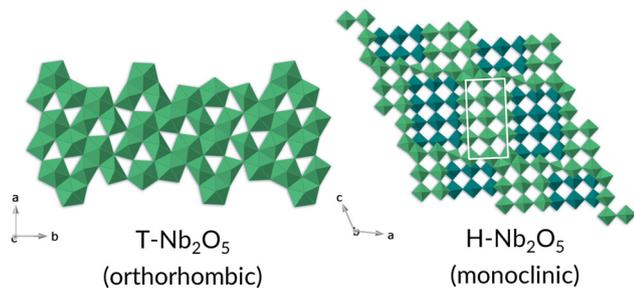
Fig. 13 Crystal structures of T- and H-Nb<sub>2</sub>O<sub>5</sub> phases, left and right respectively. The Nb is represented by the polyhedra; for simplicity the oxygens have been omitted.
