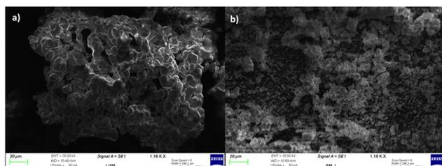
Fig. 5 SEM images of  $\text{Li}_2\text{MoO}_4$  – pristine (a) and ball milled (b).
