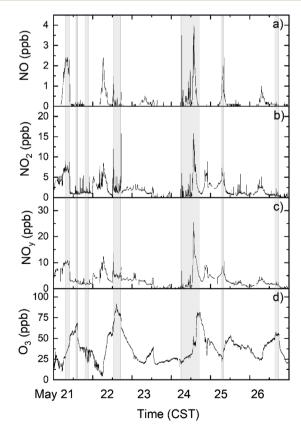
Fig. 3 Air quality ground station observations of (a) NO (ppb), (b) NO<sub>2</sub> (ppb), (c) NO<sub>v</sub> (ppb) and (d) O<sub>3</sub> (ppb) at Chiwaukee Prairie from May 21– 26, 2021. Lake breeze or onshore flow from SSE is highlighted as grey bars
