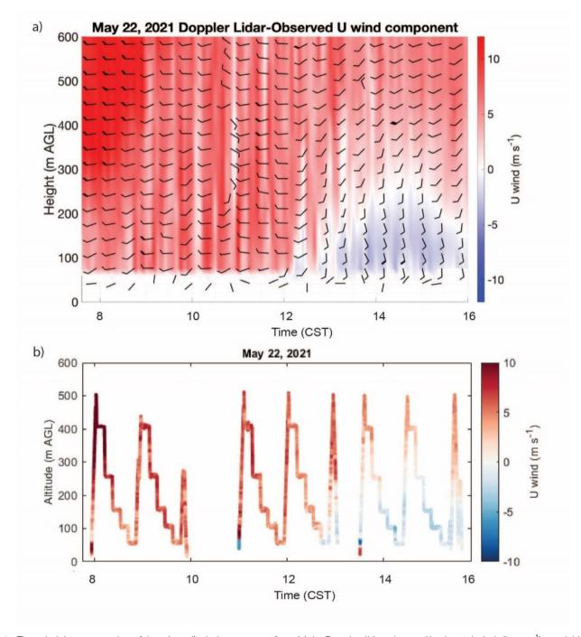
Fig. 4 Time-height cross section of the u (zonal) wind component from (a) the Doppler-lidar-observed horizontal winds (in m s<sup>-1</sup>), overlaid with horizontal wind barbs (in knots) plotted from 22 May 2021. Wind barbs are thinned by a factor of 5 in the time dimension and a factor of 2 in the height dimension to aid readability and (b) RAAVEN platform observations collected over land on May 22, 2021. In (a) is reprinted from Earth System Science Data with permission.32
