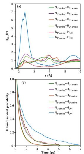
Fig. 2 (a) Partial radial distribution functions between N and H involving each type of N-H hydrogen bond potentially present in the partially PO-functionalized liquid TETA, and (b) their survival probability averaged over all hydrogen bonds of the same type from the DPMD trajectory.
