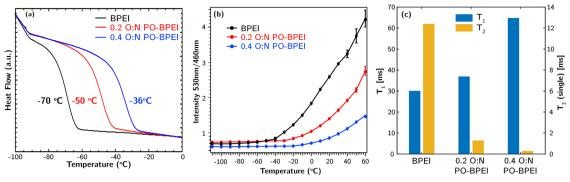
Fig. 4 (a) DSC traces and estimated  $T_0$  values, (b) temperature dependence of the ratiometric fluorescence intensity (530 nm/460 nm) with 0.5 wt% THPE dissolved in, and (c) NMR relaxometry ( $T_1$  and  $T_2$ ) for BPEI, 0.2 O:N PO-BPEI, and 0.4 O:N PO-BPEI.
