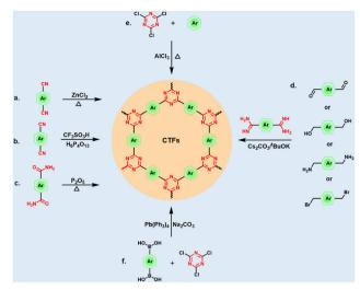
Fig. 2 Synthetic reactions and routes for the preparation of CTFs, including ionothermal method, superacid-catalyzed trimerization,  $P_2O_5$ -catalyzed method, strong base-catalyzed polycondensation, Friedel-Crafts reactions and C-C coupling reactions
