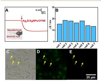
Fig. 3 (A) OCP response recorded by the Ag<sub>2</sub>S/AgNPs/CFNE inserted into a SH-SY5Y cell. Inset is a bright-field image of a SH-SY5Y cell penetrated by the  $Ag_2S/AgNPs/CFNE$ . (B) The OCP responses for measurement of endogenous H<sub>2</sub>S under the same conditions as in A. Bright-field image (C) and fluorescence image of SH-SY5Y cells stained with Calcein-AM (green, D) and PI (red, E) after penetration by the Ag<sub>2</sub>S/AgNPs/CFNE for about 100 s indicated by yellow arrows.
