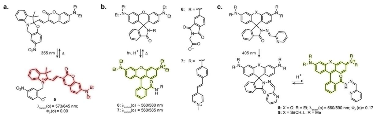
Fig. 3 (a–c) Representative structures of photoswitchable fluorophores based on a change of electronic conjugation of a fluorophore. The properties reported were measured in: MeCN for **5**; H<sub>2</sub>O for **6**; MeCN:H<sub>2</sub>O 1:1 containing acid for **7**; aqueous buffer pH = 5 for **8**. The notation (o) refers to the open isomer.
