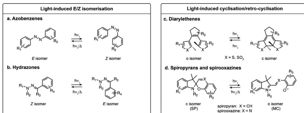
Fig. 1 Representative structures and photoisomerisation of most common classes of photoswitches applied in fluorescence microscopy. R<sub>1</sub>–R<sub>4</sub> indicate the most frequent substitution positions.
