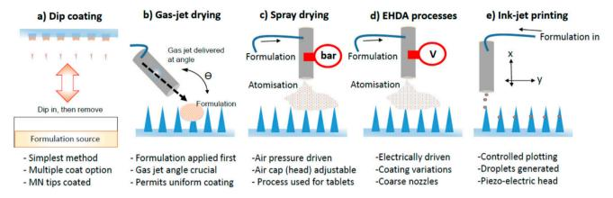
Fig. 3 Illustrated examples of techniques used to coat MNs. (a) Dip coating; (b) gas-jet drying; (c) spray drying; (d) EHDA processes; (e) ink-jet printing. Reprinted with permission from MDPI,<sup>20</sup> Copyright 2015.
