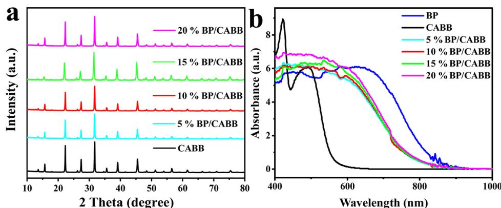
Fig. 2 (a) XRD and (b) DRS patterns of the obtained CABB, BP and BP/CABB.
