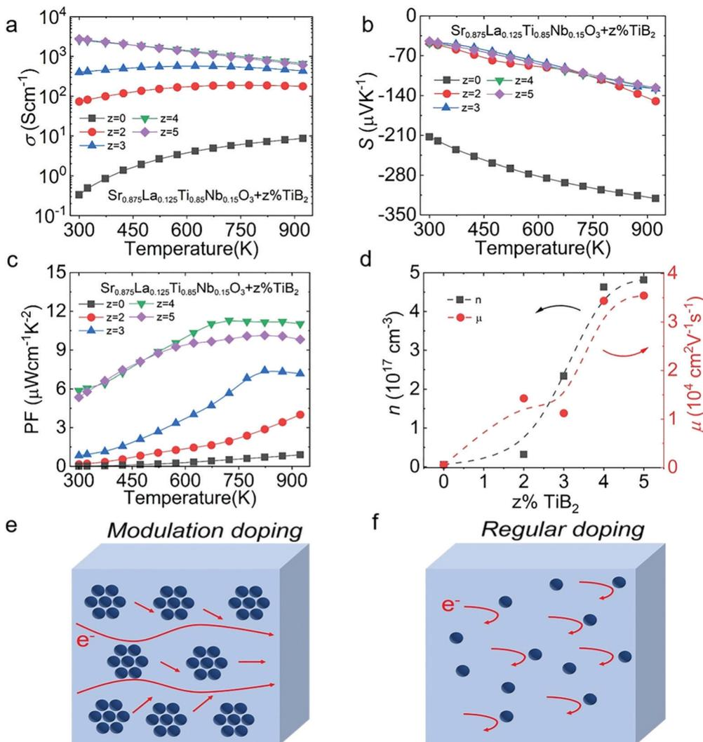
Fig. 9 Electrical transport properties for  $\text{Sr}_{0.875}\text{La}_{0.125}\text{Ti}_{0.85}\text{Nb}_{0.15}\text{O}_3 + z\% \text{TiB}_2$  ( $z = 0-5$ ): (a)  $\sigma$ ; (b)  $S$ ; (c) PF; (d)  $n$  and  $\mu$ . (e) Modulation-doped semiconductor and (f) regular doped semiconductor.
