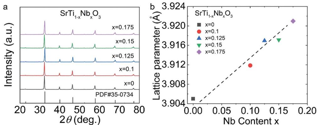
Fig. 3  $\text{SrTi}_{1-x}\text{Nb}_x\text{O}_3$  ( $x = 0-0.175$ ): (a) XRD patterns and (b) lattice constant.
