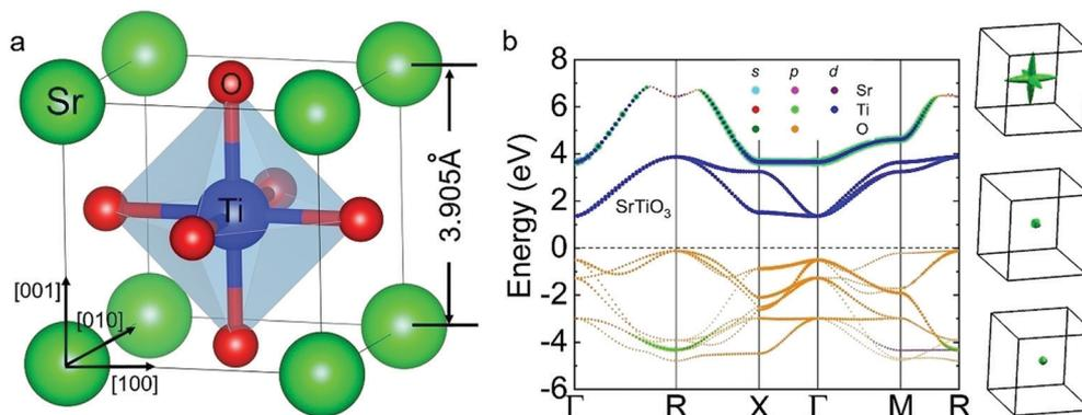
Fig. 1 Structural characterization of SrTiO<sub>3</sub>: (a) structure of the crystal and (b) the atomic orbital resolved electronic band structure. The triple degenerate CBM is located at the  $\Gamma$  point. The right panel shows the Fermi energy surface in the first-Brillouin zone with the isosurface level  $E_{\text{CBM}} + 0.05$  for these three degenerate bands.
