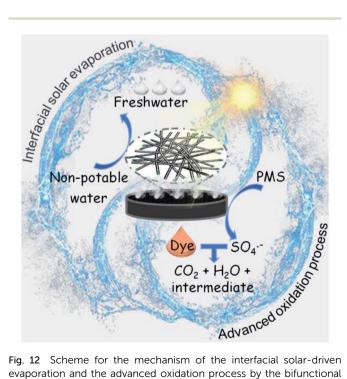
Fig. 12 Scheme for the mechanism of the interfacial solar-driven evaporation and the advanced oxidation process by the bifunctional NC-700 evaporator under visible light irradiation.
