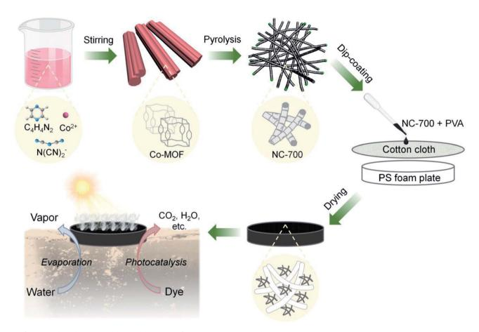
Fig. 1 Scheme of the fabrication of the bifunctional NC-x evaporator for interfacial solar-driven evaporation and the photocatalytic degradation of organic dyes (note: x stands for the calcination temperature, e.g., 700 °C; after coating, the PS foam plate was covered by the black NC-x evaporator).
