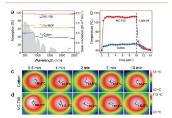
Fig. 5 (a) UV-Vis-NIR absorption spectra of cotton, Co-MOF and the NC-700 evaporator. (b) Surface temperature curves, and (c and d) infrared images of cotton and the NC-700 evaporator under 1 sun irradiation.
