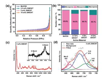
Fig. 3 BET analyses of MnVOH, 2.5 wt% SWCNTs, 5 wt% SWCNTs, and 10 wt% SWCNTs: (a) N2 adsorption—desorption isotherms; (b) BET surface area. Raman spectrum: (c) 5 wt% SWCNTs (inset is the spectrum from 1200 to 1700 cm $^{-1}$ ), and (d) partially fitted spectra to show the presence of the Mn-O bond.
