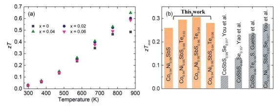
Fig. 6 zT value of the  $Co_{0.94}Ni_{0.06}SbS_{1-x}Te_x$  samples (x=0, 0.02, 0.04, and 0.06). (a) Temperature-dependent zT values and (b) comparison of the  $Co_{0.94}Ni_{0.06}SbS_{1-x}Te_x$  samples with other reported CoSbS samples prepared by Hou et al., Yao et al., and Guelou et al.
