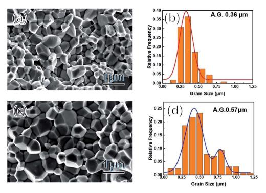
Fig. 3 (a and c) SEM images of freshly fractured surfaces of  $Co_{0.94}Ni_{0.06}SbS$  and  $Co_{0.94}Ni_{0.06}SbS_{0.96}Te_{0.04}$ , respectively; (b and d) their corresponding grain-size distribution analysis.
