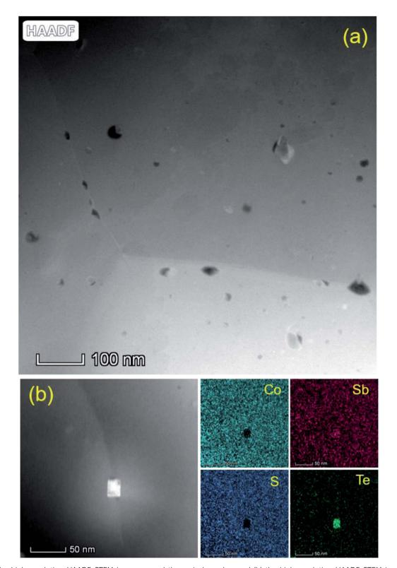
Fig. 4 (a) The high-resolution HAADF-STEM image around the grain boundary and (b) the high-resolution HAADF-STEM image and EDS mapping of the elemental segregation along the grain boundary.
