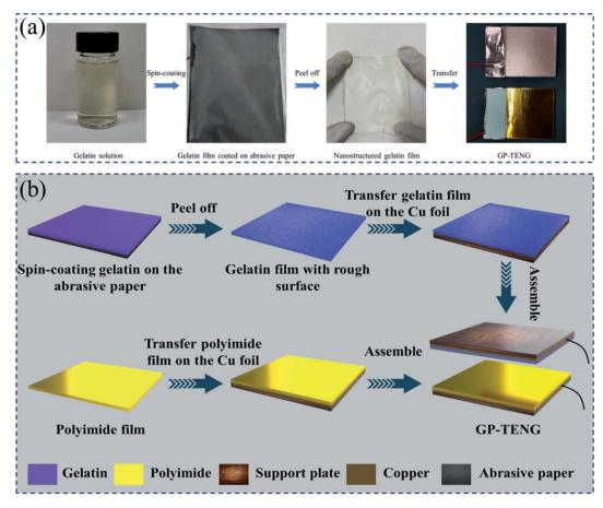
Fig. 1 (a) The preparation flow chart of the nanostructured gelatin film with abrasive paper as the template. (b) The assembly flow chart of the GP-TENG.
