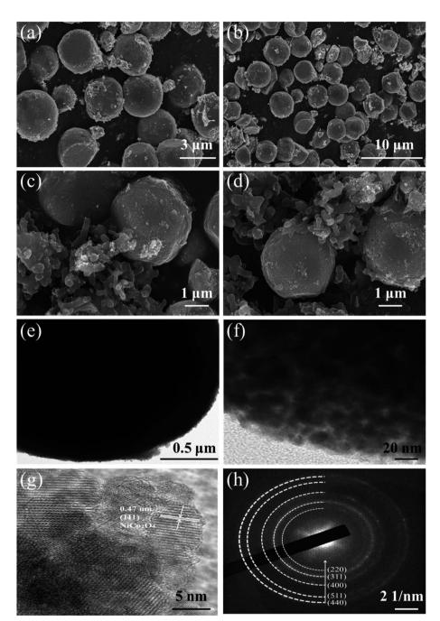
Fig. 5 SEM images of (a and b) NiCo<sub>2</sub>O<sub>4</sub> nanospheres at different scales. (c and d) The PANI/NiCo<sub>2</sub>O<sub>4</sub> composite. TEM images of (e and f) NiCo<sub>2</sub>O<sub>4</sub> nanospheres at different magnifications. (g) HRTEM images of NiCo<sub>2</sub>O<sub>4</sub> nanospheres. (h) The corresponding SAED pattern of NiCo<sub>2</sub>O<sub>4</sub> nanospheres.
