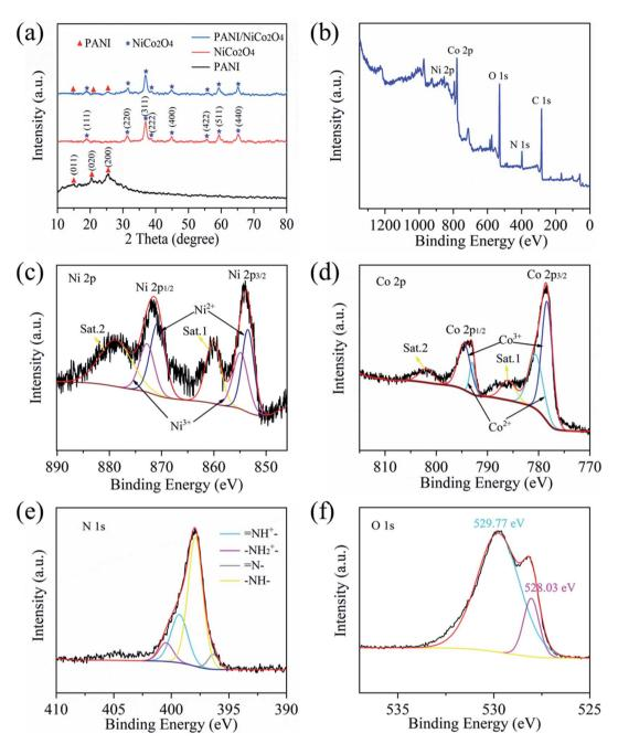
Fig. 6 (a) XRD pattern of pure PANI, pure NiCo<sub>2</sub>O<sub>4</sub> and the PANI/NiCo<sub>2</sub>O<sub>4</sub> composite. XPS spectra of the PANI/NiCo<sub>2</sub>O<sub>4</sub> composite: the (b) survey spectrum, (c) Ni 2p spectrum, (d) Co 2p spectrum, (e) N 1s spectrum and (f) O 1s spectrum.
