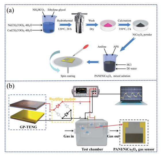
Fig. 2 (a) The diagram of preparation process of the  $NH_3$  gas sensor based on the  $PANI/NiCo_2O_4$  composite. (b) The experimental test platform of the self-powered GPAS based on the  $PANI/NiCo_2O_4$  composite.
