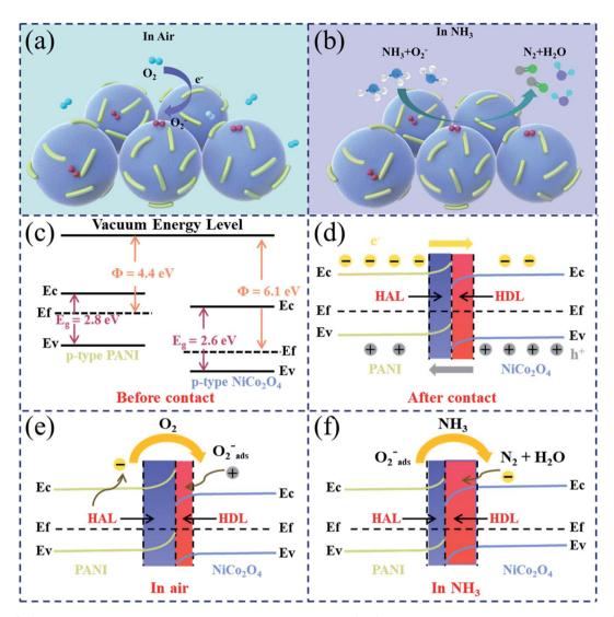
Fig. 8 (a and b) Gas adsorption and desorption processes on the surface of  $NiCo_2O_4$  nanospheres in air and  $NH_3$ , respectively. (c and d) The energy band diagram of PANI and  $NiCo_2O_4$  before and after contact, respectively. (e and f) The energy band structure of the PANI/ $NiCo_2O_4$  heterojunction exposed to air and  $NH_3$ , respectively.
