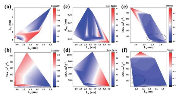
Fig. 3 Contour maps of change trends for dual structural parameters and sodium storage performance. (a and b) Capacity; (c and d) rate; (e and f) plateau.
