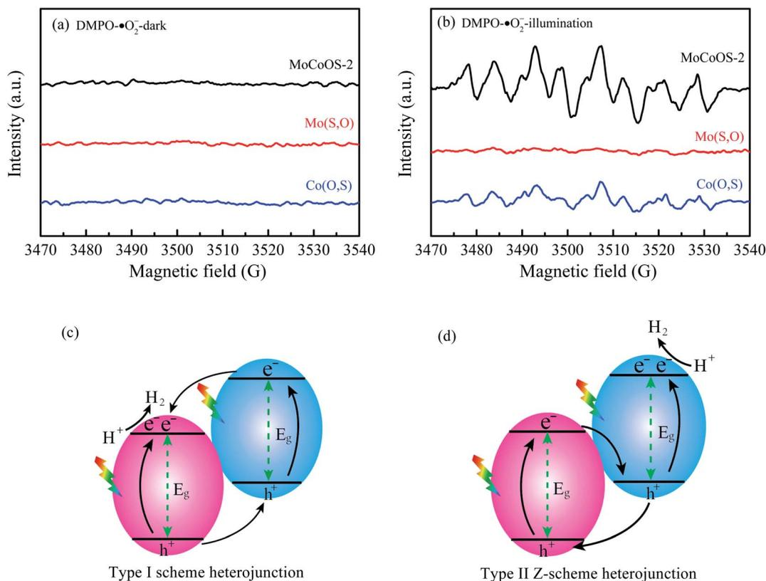
Fig. 14 EPR spectra of (a)  $\text{DMPO}-\cdot\text{O}_2^-$  and (b)  $\text{DMPO}-\cdot\text{O}_2^-$  for Mo(S,O), Co(O,S), and MoCoOS catalysts under darkness and illumination for 10 min. (c and d) The two types of heterojunction.
