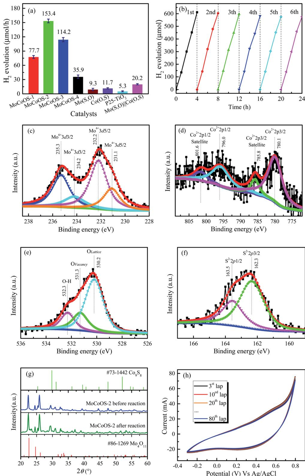
Fig. 7 (a) Hydrogen production of MoCoOS, Mo(S<sub>2</sub>O), Co(O,S), Mo(S<sub>2</sub>O)||Co(O,S) and P25-TiO<sub>2</sub> catalysts. (b) Recycling hydrogen production reaction performance of MoCoOS-2. (c-f) XPS spectra of MoCoOS-2 after the hydrogen evolution reaction. (g) XRD patterns of MoCoOS-2 before and after the hydrogen evolution reaction. (h) Cyclic voltammetry of MoCoOS-2 for 80 cycles.
