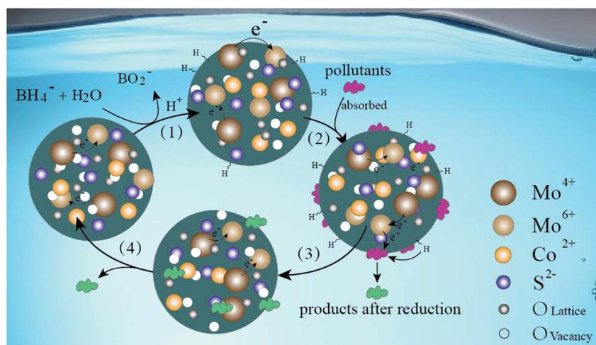
Fig. 16 The schematic reaction of organic dyes in the presence of the MoCoOS catalyst and NaBH<sub>4</sub>.
