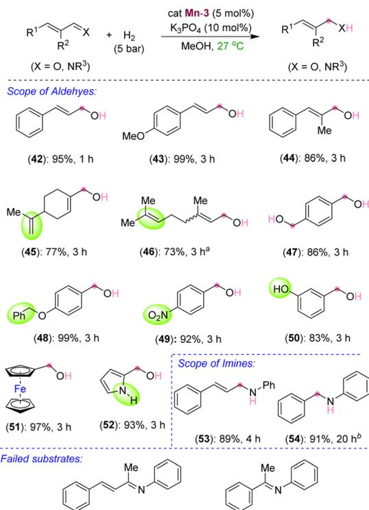
**Scheme 4** Scope of Mn-catalyzed hydrogenation of aldehydes and imines. <sup>a</sup>Reaction conditions: substrate (0.20 mmol), **Mn-3** (0.005 g, 0.01 mmol, 5 mol%), K<sub>3</sub>PO<sub>4</sub> (0.0043 g, 0.02 mmol), H<sub>2</sub> (5 bar), MeOH (1.0 mL). Yields are of isolated compounds. <sup>b</sup>Obtained as a mixture of *E* and *Z* isomers as the starting compound was also a mixture of both. <sup>c</sup>Reaction performed at 50 °C.
