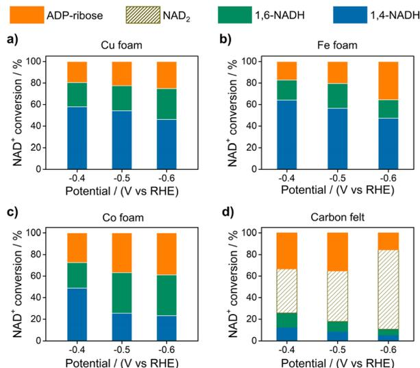
Fig. 2 The conversion of NAD<sup>+</sup> to different products on (a) Cu, (b) Fe, (c) Co foams, and (d) carbon felt at different potentials. Electrolyte: 0.1 M phosphate buffer (pH 7); catholyte: 12 mL electrolyte with an initial NAD<sup>+</sup> concentration of 1 mM.
