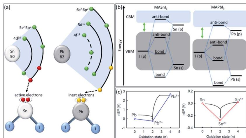
Fig. 1 (a) The electronic structure of Sn and Pb atoms. (b) Schematic energy levels of MASnI<sub>3</sub> vs. MAPbI<sub>3</sub> perovskites. (c) Frost diagrams of different oxidation states for Pb and Sn elements.<sup>47</sup> Copyright 2021, American Chemical Society.
