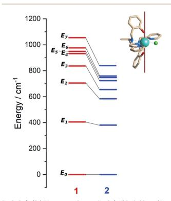
Fig. 2 Left: *Ab initio* computed energy levels for **1** (red, this work) and **2** (blue, Tong and co-workers ref. 22). Each bar represents a Kramers doublet. Right: structure of **1** showing the direction of the ground Kramers doublet magnetic easy axis. Color code: cyan/Dy, green/Cl, blue/N, red/O, khaki/C. Hydrogen atoms are omitted for clarity.
