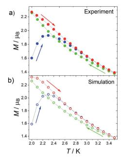
Fig. 6 (a) Experimental and (b) simulated ZFC (blue) and FC (green and red) curves of 1 at a sweeping rate of  $0.03 \, \text{K s}^{-1}$  and at  $H = 1.6 \, \text{kOe}$ . The arrows indicate the direction of the measurement for each curve.
