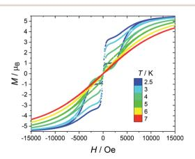
Fig. 5 Temperature dependence of the hysteresis loops of 1. Field sweeping rate:  $100 \text{ Oe s}^{-1}$ .
