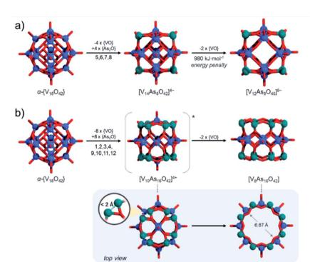
Fig. 12 Schematic juxtaposition of (a) substitution of four  $[VO]^{2+}$  sites in the central belt of  $\alpha$ - $\{V_{18}O_{42}\}$  leading to energetically unfavourable further  $2 \times [VO]^{2+}$  loss; (b) substitution of eight  $[VO]^{2+}$  sites of the two cupolaed in  $\alpha$ - $\{V_{18}O_{42}\}$  leading to geometrically favourable  $2 \times [VO]^{2+}$  loss. Colour code: V = blue, As = green, and O = red spheres.
