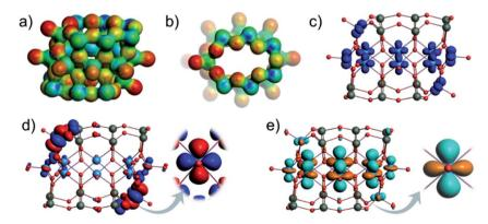
Fig. 15 Molecular electrostatic potential (MEP) plotted over the density isosurface of  $[V_{10}As_{12}O_{40}]^{4-}$  shown in (a) side and (b) top view. The most negative potentials are shown in red. Spin density isosurfaces indicating accumulation of  $\alpha$  spins for  $[V_{10}As_{12}O_{40}]^{4-}$  (c). Depiction of the HOMO (d) and the LUMO of  $[V_{10}As_{12}O_{40}]^{4-}$  (e). Colour code: V = blue, O = red, and O = red, and O = red.
