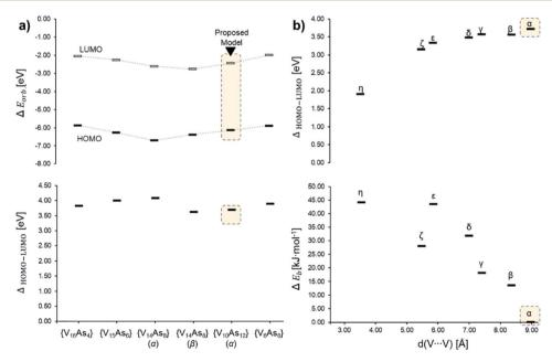
Fig. 14 Energy diagrams based on Tables S7 and S8,† showcasing (a) the α-spin HOMO and LUMO (top) and HOMO-LUMO gap (bottom) energies among different experimentally described As-POVs and the herein proposed  $\alpha$ -[ $V_{10}$ As<sub>12</sub>O<sub>40</sub>]<sup>4-</sup> model; (b) HOMO-LUMO gap (top) and relative bonding energy in of the isomeric  $[V_{10}As_{12}O_{40}]^{4-}$  in comparison to the  $\alpha$ -structure.
