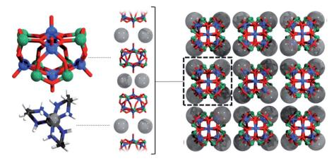
Fig. 3 Ball and stick representation of an individual  $[V_6As_8O_{26}]^{4-}$  polyanion and the  $[Ni(en)_3]^{2+}$  dications (left), followed by their hierarchical packing from one (middle) to three dimensions (right). Colour code: V = blue, O = red, As = green, N = dark blue, Ni = grey, C = black, H = white spheres. For clarity,  $[Ni(en)_3]^{2+}$  in the middle and right figure are represented as transparent grey spheres.
