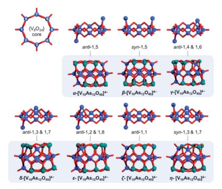
Fig. 13 Enumeration of the eight V centres in the  $\{V_8O_{24}\}$  cores deriving from the  $[V_8As_{16}O_{40}]$  structure (top left), followed by the depiction of substitution patterns and the respective  $[V_{10}As_{12}O_{40}]^{4-}$  isomers positioned in the shaded box areas colour code: V = blue, O = red, and As = colourgreen spheres.
