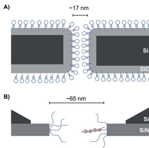
**Fig. 11** Solid-state nanopores modified using 1,4-phenylene diisothiocyanate as a cross-linking agent to attach amino-terminated (A) DNA hairpins<sup>56</sup> and (B) single-stranded DNA.<sup>57</sup> The passage of complementary strands through such pores was slowed, resulting in prolonged ion current drops.
