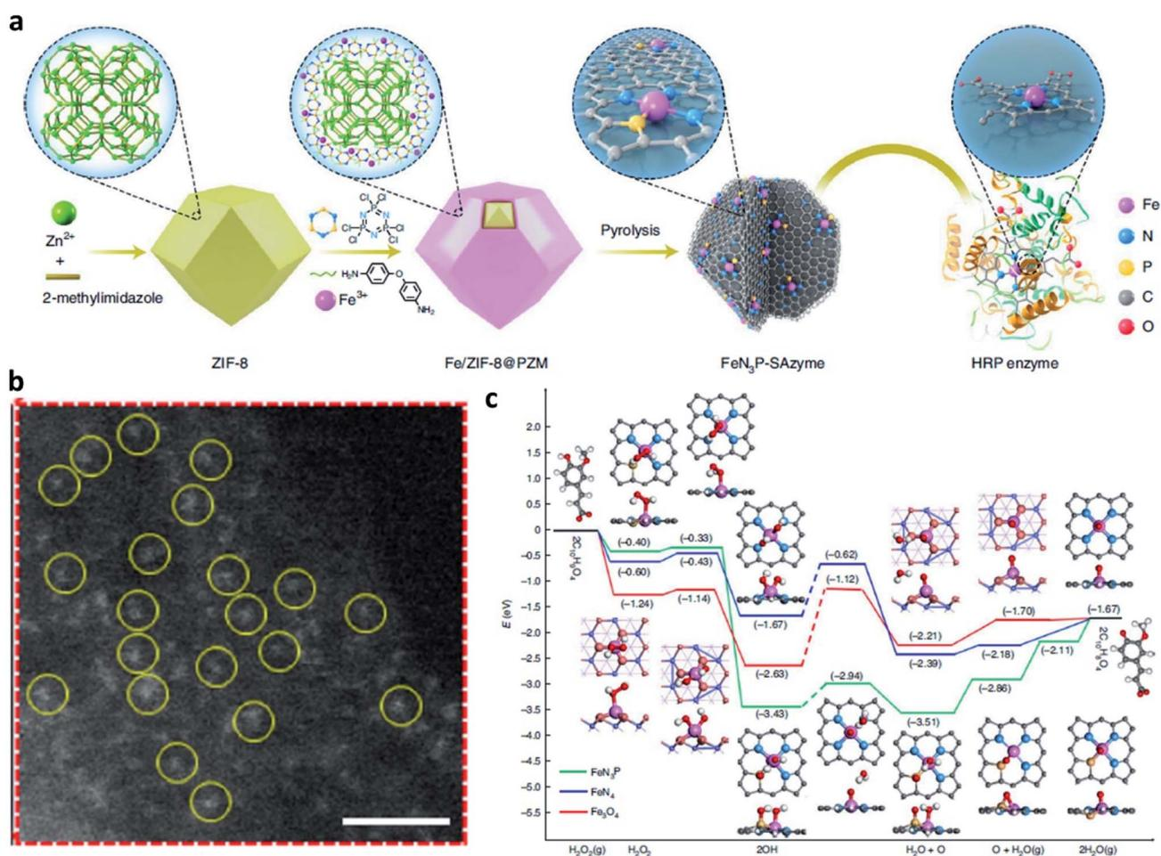
Fig. 11 (a) Schematic synthetic process of FeN<sub>3</sub>P-SAzyme (SAzyme: single-atom nanozyme). (b) AC HAADF-STEM image of FeN<sub>3</sub>P-SAzyme. Scar bar: 1 nm. (c) DFT calculations on the POD-like activity of FeN<sub>3</sub>P-SAzyme, FeN<sub>4</sub>-SAzyme, and Fe<sub>3</sub>O<sub>4</sub> nanozyme for comparison. Color code: C, grey; Fe, blue; N, light blue; O, light red; P, yellow; H, white. Reproduced with permission from ref. 57. Copyright 2021, Nature Publishing Group.
