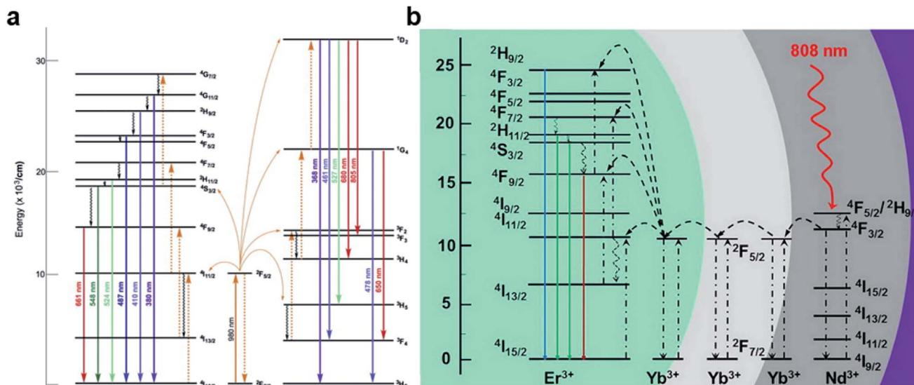
Fig. 1 Proposed energy transfer mechanism showing the UCL processes in (a)  $\text{Er}^{3+}$ ,  $\text{Tm}^{3+}$ , and  $\text{Yb}^{3+}$  doped UCNP under 980 nm laser excitation<sup>31</sup> and (b)  $\text{Nd}^{3+}$ ,  $\text{Yb}^{3+}$ , and  $\text{Er}^{3+}$  doped UCNP under 808 nm laser excitation.<sup>32</sup> Adapted from ref. 31 with permission from Elsevier Ltd, copyright 2014; adapted from ref. 32 with permission from American Chemical Society, copyright 2016.
